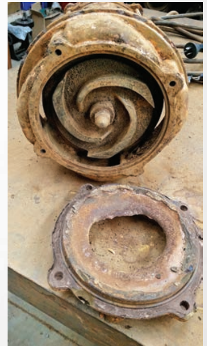
The 'high chrome' impeller was in excellent condition but the suction cover plate was understandably worn
