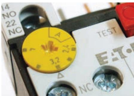
Rotate the yellow dial to match the full load amps of the motor.
