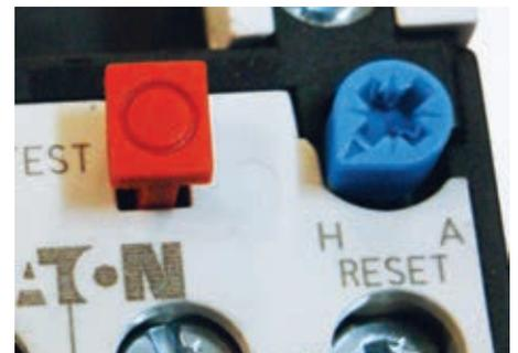
Controls like the small blue dial above should be on manual reset.
