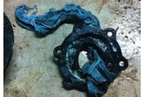
After jamming a sewage pump, this rag was removed, the thermal overload was reset and the pump operated normally again.
